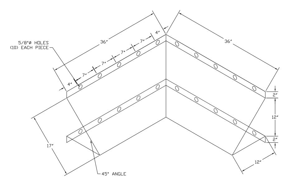
PLEASE NOTE: MADE OF ALUMINIZED OR GALVANIZED STEEL.
